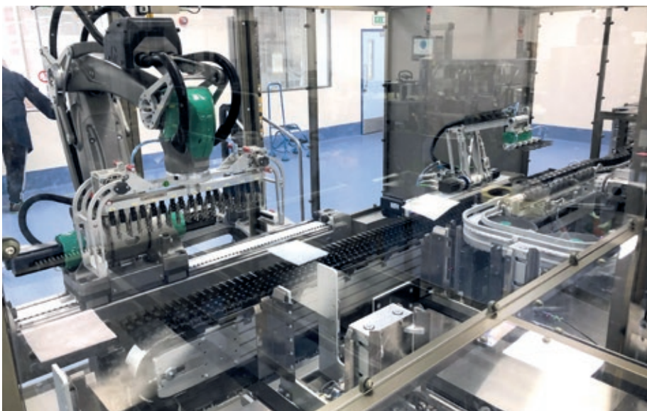
Figure 1: The Gigacombi (left) empties trays and stacks empty trays, and the Robocombi (right) inserts devices into pucks for downstream packaging.
