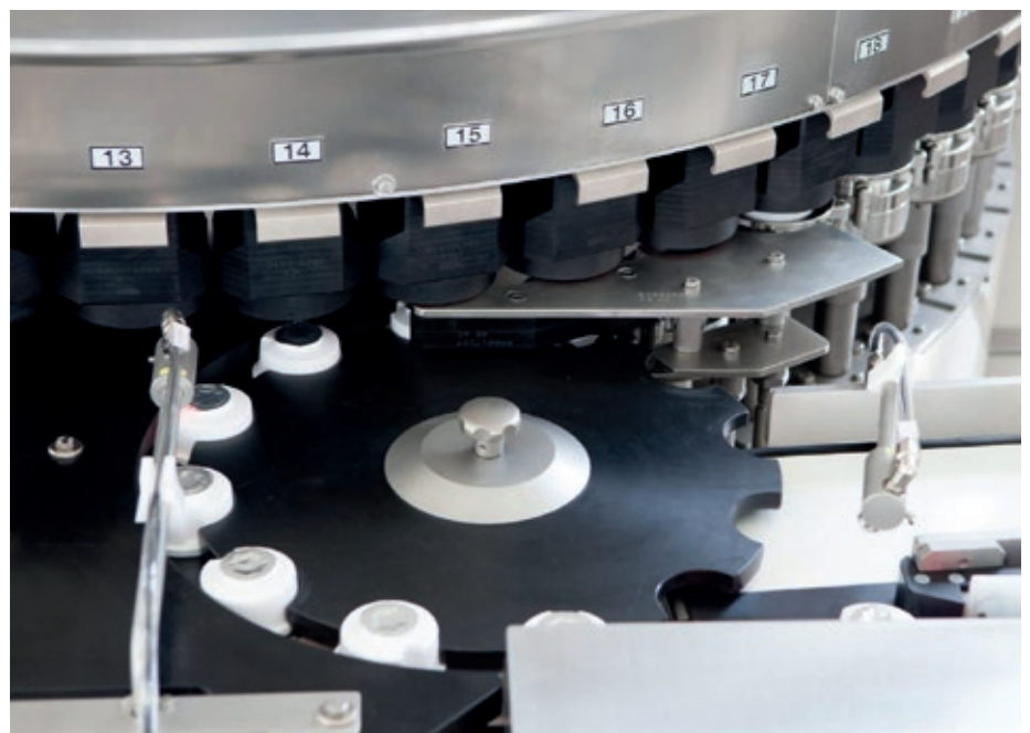
Figure 5: Image of an in-line vacuum decay CCIT method used during production. Photo courtesy of Bonfiglioli Engineering Srl.
